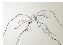
The test kit is equilibrated to room temperature, take samples by capillary in front of the sample collector, insert the sample collector into the cuvette.
