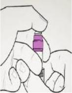
Inject the reagent R2 into the cuvette.
